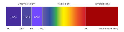
UVC light has been used for disinfection in industry and in hospitals for many years. UVC light has a wavelength of 253.7 nm and is therefore invisible to the human eye.
