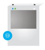
If the blue and green LED lamps light up at the same time, zero the box by holding both hands over the two sensors at the same time for 10 seconds.
