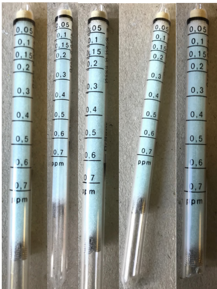
Figure 1: Short-term tubes after measurements in the following order from left to right: Unused tube, background measurement, measurements during use of the UV box, cycle 1-3.
